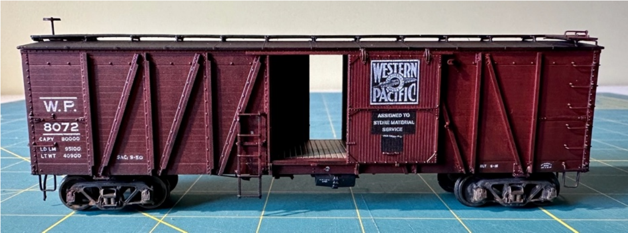
Stores (Company Material) car. 2 styles of ladders are provided. Note no dimensional data.
