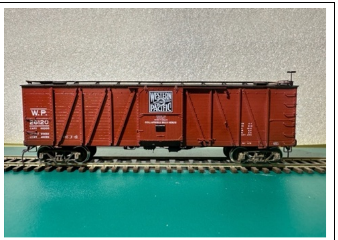
Gypsum car converted in 1942, 4 hatch version.
