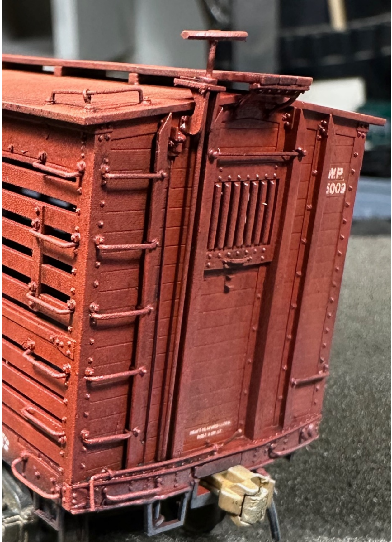
Typical end detail. For Stockcars, note the 2nd from bottom grab on the sides and the Drover door grab bar. (the brakewheel is too low, should be 15" above fitting)
