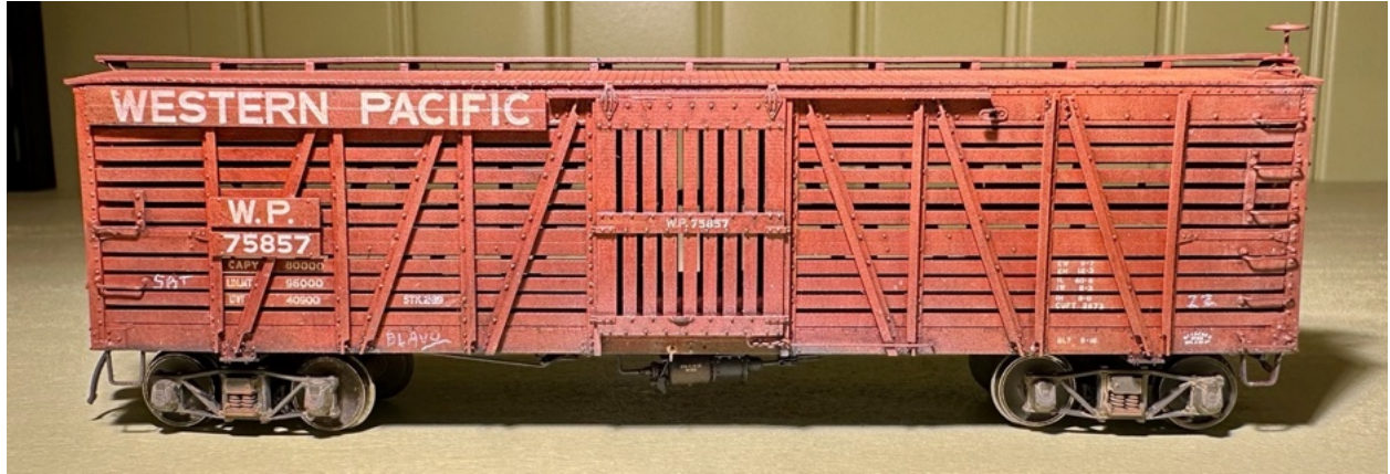
Early stockcar version with wood roof and roadname/number boards. Archbar trucks when converted, replaced by Andrews in the '50's.
