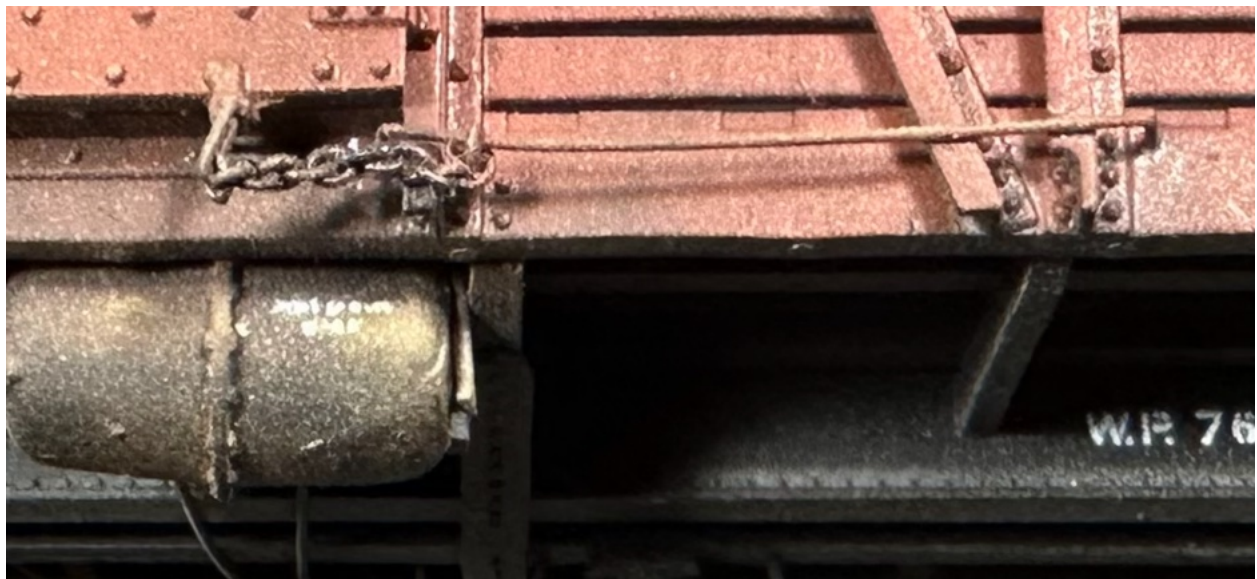
Showing Stockcar door rail detail. Underframe car numbers on the right.
