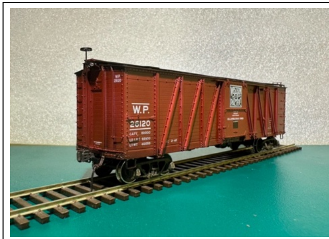
Gypsum car converted in 1942, 4 hatch version.
