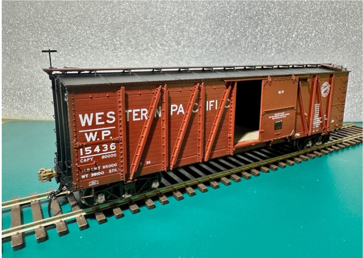
How a typical post 1927 ARA lettering would have looked from the late 1930s until 1948, pre-weathering. The last prior time it would have been painted was in that 1927-1930 timeframe until being stencilled for online use only in prep for the July 1940 interchange limitation.
