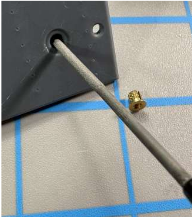
Cleaning hole to accept brass insert to be press fit with a small rat tail file
