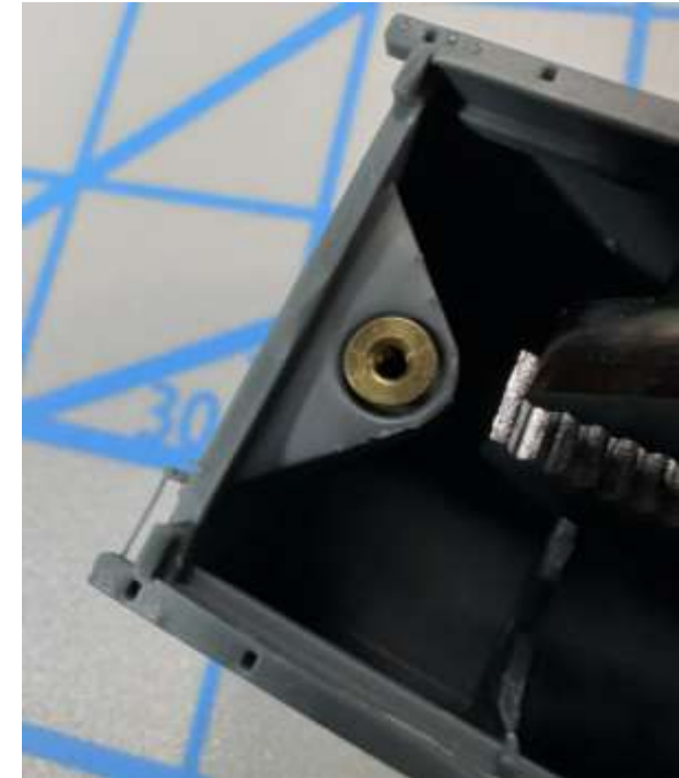
Brass insert properly pressed/inserted in hole
